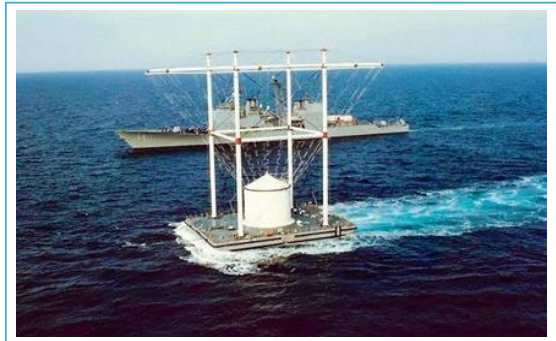
Figure 27. EMP test scene for naval vessels[17]
