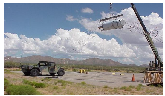
Figure 26. EMP test scene for ground vehicle[16]
