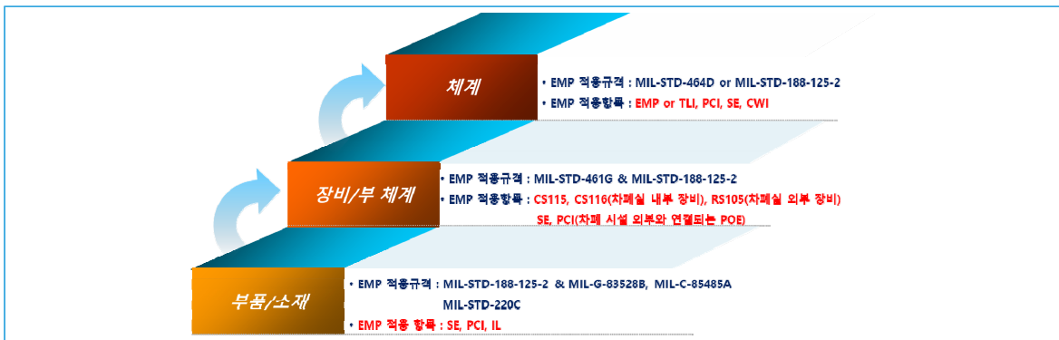
Figure 28. Step-by-step EMP application standards and items for weapon systems[8]
